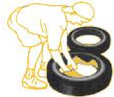
Wall framing using automotive tyres
